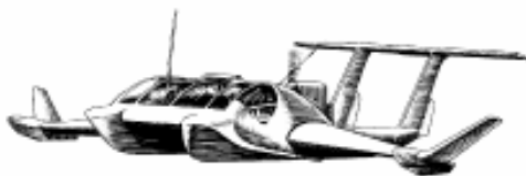
Figure 35: Hoverwing-20 with a static air-cushion lift-off system [22]
