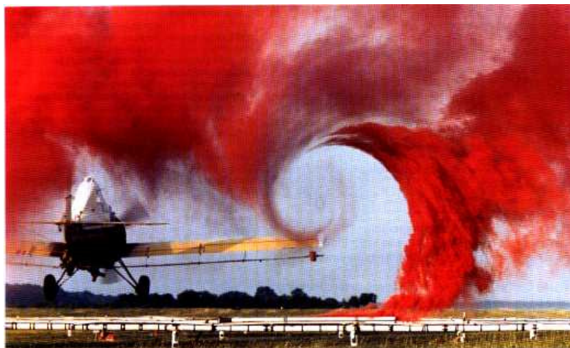
Figure 1: Vortices on the tip of a wing [33]
