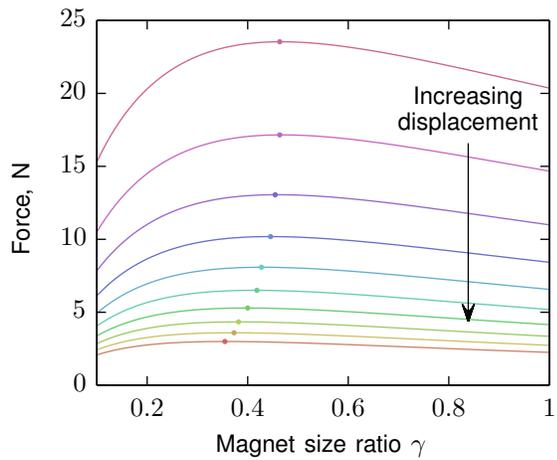
Fig. 4: Force between two magnets as a function of magnet height–width ratio  $\gamma = a/b$  at a number of fixed displacements from 1 mm to 10 mm. The positions of maximum force are shown with dots, indicating that magnet size ratio to achieve the maximum force is in the region around  $\gamma = 0.4$ .
