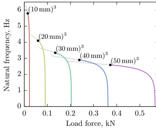
Figure 7: Natural frequency versus load force for a magnet gap ratio of 0.2 and a magnet angle of  $40^\circ$  over a range of magnet volumes from  $(10 \text{ mm})^3$  to  $(50 \text{ mm})^3$ . The displacement ranges are proportional to the magnet size such that the system with magnet volume  $(10 \text{ mm})^3$  undergoes displacement from 0 mm to 10 mm and the system with volume  $(50 \text{ mm})^3$  moves over 0 mm to 50 mm. Regions of negative horizontal stiffness are drawn in light gray.
