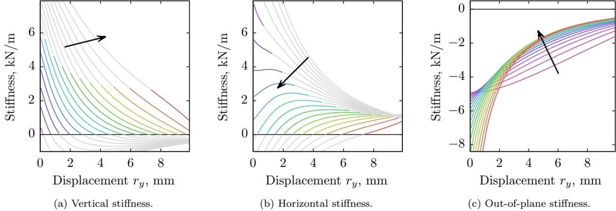
Figure 5: Stiffness in three directions versus displacement for a gap ratio of 0.2 and magnet angles from  $0^\circ$  to  $90^\circ$  in  $5^\circ$  increments (arrows indicate increasing magnet angle). For the horizontal and vertical stiffness plots (a) and (b), regions of positive stiffness for both directions are coloured; regions of gray indicate that either the vertical and/or horizontal stiffness is negative in that position for that magnet angle.
