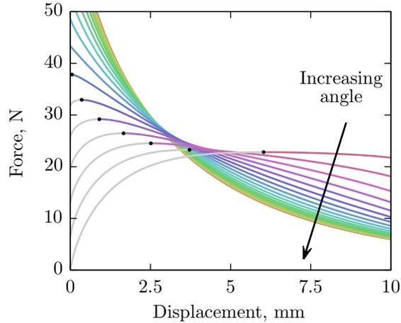
Figure 2: Force versus displacement for magnet angles from  $0^\circ$  to  $90^\circ$  in  $5^\circ$  increments. The offset distance between the magnets is zero. Light gray lines indicate negative stiffness (instability) and markers show the position of quasi-zero stiffness.
