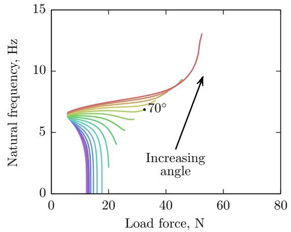
(b) Gap ratio of 0.25. Near-constant natural frequency occurs at  $70^\circ$ .
