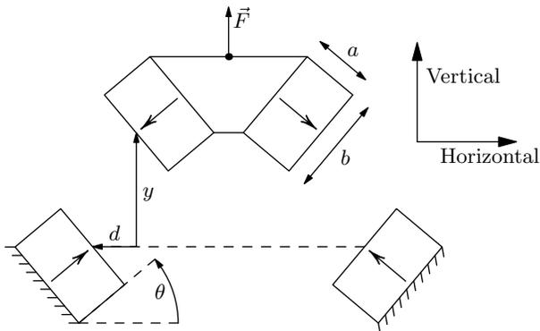
Figure 1: Schematic of the oblique-magnet spring. When magnet offset  $d = 0$  and displacement  $y = 0$ , the magnet faces are aligned and touching. Displacements  $x$  and  $z$  (not shown) are in the horizontal and out-of-plane directions, respectively.
