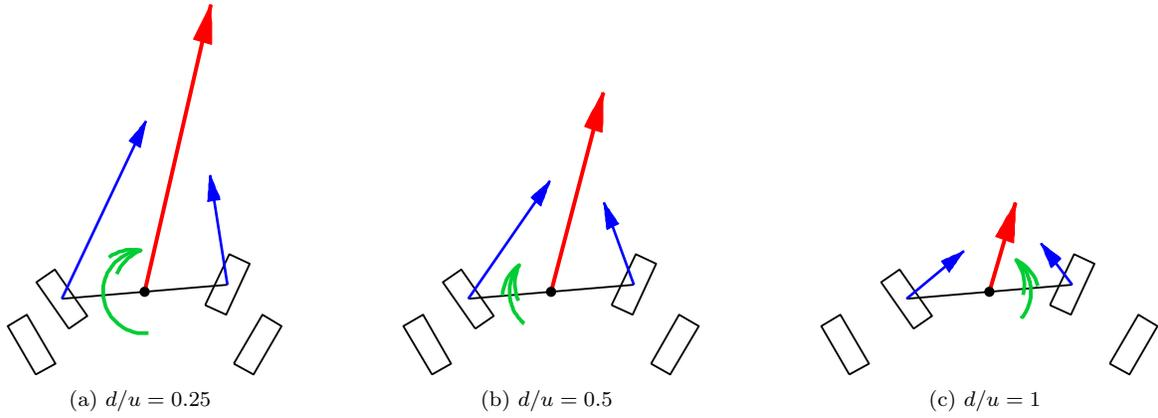
Figure 11: Visual representation of the forces and torques at a rotation of  $\varphi = 10^\circ$  corresponding to the stability results shown in Fig. 10. Force vector lengths are proportional to their magnitude, but torque arc lengths are not.
