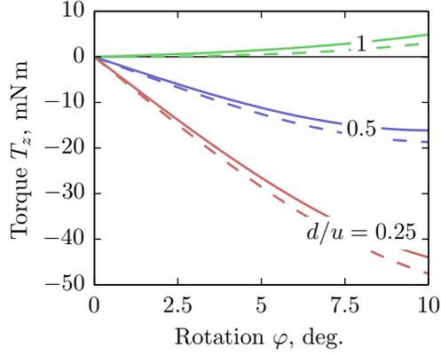
Figure 10: Torque versus rotation for a certain spring configuration with parameters  $u = y = 10$  mm,  $\theta = 30^\circ$ , and  $l/u = 2$ . Dashed lines show for verification torque as if calculated using the magnetic forces around their lever arms only (Eq. (13)). Notice that varying the magnet gap ratio (shown) can vary the rotational stiffness from stable ( $d/u = \{0.25, 0.5\}$ ) to unstable ( $d/u = 1$ ). Geometries for these three configurations are shown in Fig. 11.
