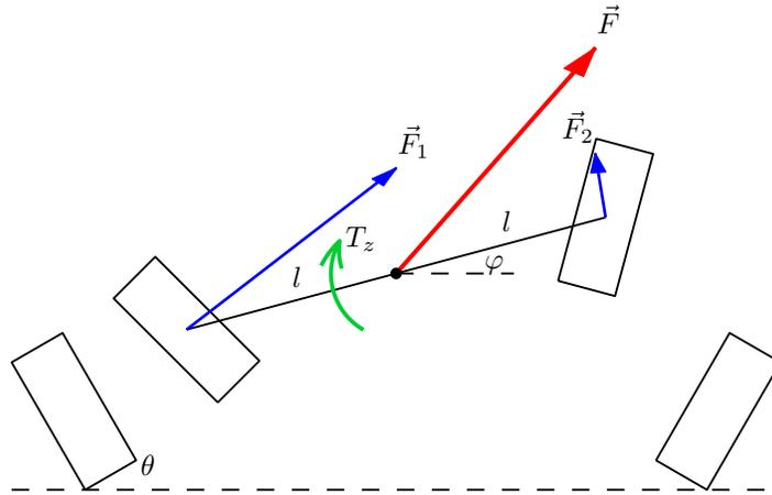
Figure 8: Geometry of the planar system in which forces and torques due to rotation  $\varphi$  are calculated. The system is shown with  $\varphi = 15^\circ$ , lever arm ratio  $l/u = 2$ , magnet angle  $\theta = 30^\circ$  and magnet gap ratio  $d/u = 0.5$ .
