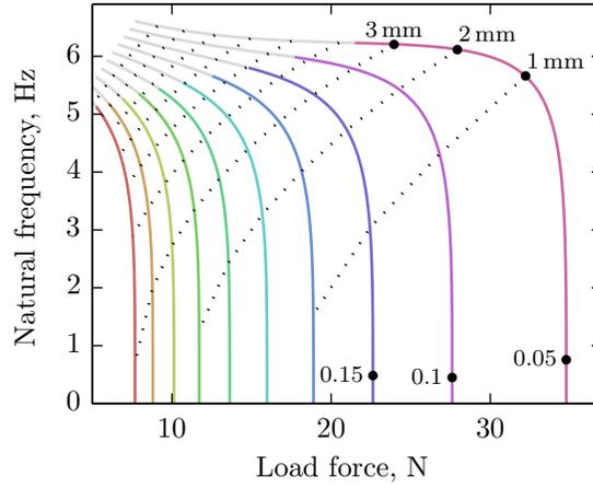
Figure 6: Natural frequency versus load force for gap ratios from 0.05 to 0.5 in 0.05 increments and a magnet angle of  $40^\circ$ . Regions of negative horizontal stiffness are drawn in light gray, and displacements are labelled with dotted lines for every change in displacement of 1 mm.
