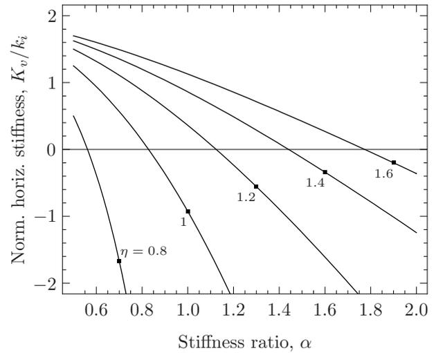
**Figure 5.** Horizontal stiffness characteristic at the vertical quasi-zero stiffness condition for varying stiffness ratio  $\alpha$  and length ratio  $\eta$ , calculated with Eq. (20).
