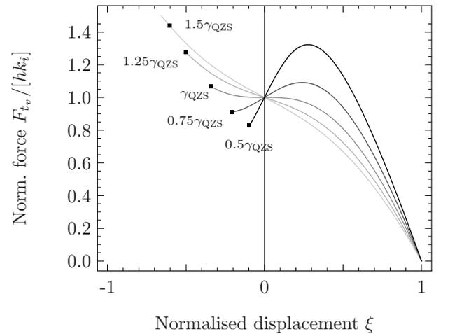
(b) Normalised vertical force characteristic of the system calculated with Eq. (8). Minimum displacements are calculated from Eq. (9); these termination points represent the limiting case of the vertical spring being compressed to zero length.
