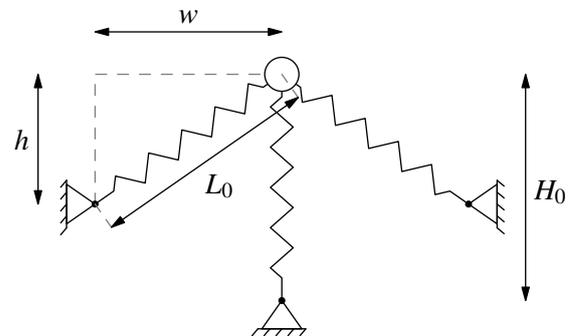
(a) Inclined springs in their uncompressed state, corresponding to a vertical displacement of  $z = h$ .
