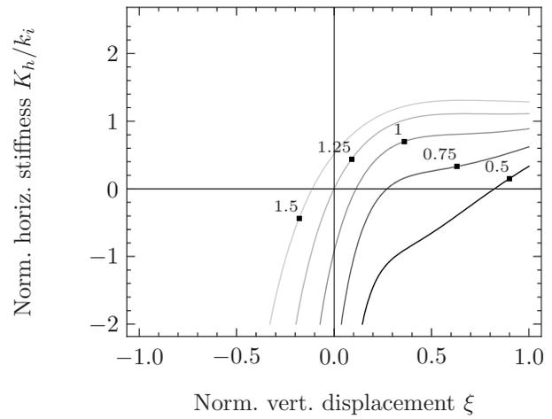
(b) Normalised horizontal stiffness of the system calculated with Eq. (19).
