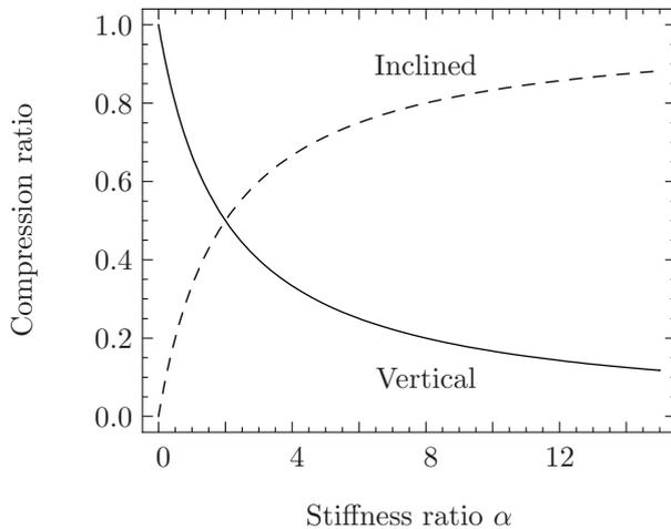
**Figure 8.** Compression relationship of the springs for a range of spring stiffness ratios, at quasi-zero stiffness both horizontally and vertically. A compression of 100% implies a change in displacement of the entire spring length, which is difficult to realise in practice.
