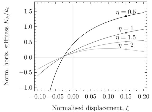
**Figure 7.** Normalised horizontal stiffness of the system at  $\alpha = 0.95\alpha_{QZS}$  in order to obtain a small range of displacement around  $\xi = 0$  with positive stiffness (compare with Figure 6b which has negative stiffness for  $\xi < 0$ ). The vertical quasi-zero stiffness condition is unaffected.
