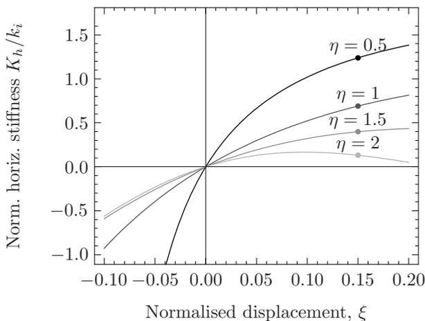
(b) Normalised horizontal stiffness of the system; negative displacement will result in negative stiffness.
