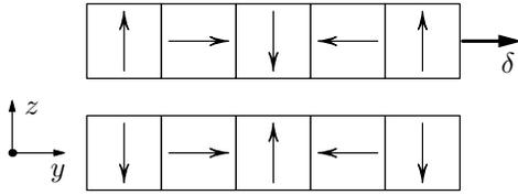
Fig. 6: Multipole system composed of 10 mm cube magnets for  $\delta = 0$ . Forces in the  $y$ - and  $z$ -directions as  $\delta$  varies are shown in Figure 7.
